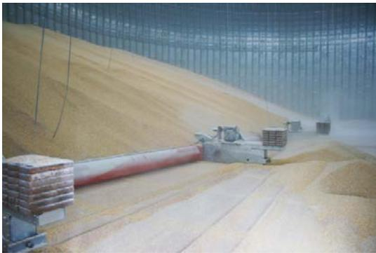
this a bin sweep it is found inside a grain bin and moves around the bin floor to move the grain to a central sump (a pit under the bin that has another auger that then moves the grain away and onto to truck) The components of the bin sweep may not be guarded and can quickly entangle a person who may come in contact with the sweep. Typically the sweep is control by a switch on the outside of the bin.
