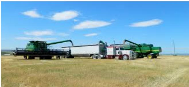
grain trucks vary from 'semi's' , which are load from the top and unloaded via hoppers at the bottom.
