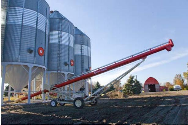
Hopper bottom grain bins, machine in the foreground is a grain auger it can be used either for filling or emptying a grain bin
