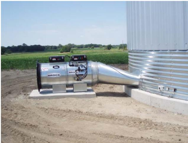
grain bin aeration systems blow air from the outside into the bin through a series of ducts to cool the grain and remove moisture from the kernels of grain.
