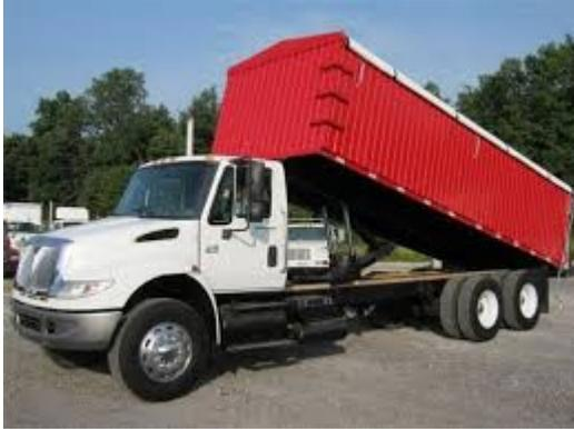
to tandem trucks that have a box that is hoisted to 'pour' the grain out the back.
