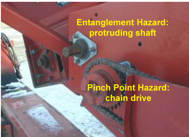
Figure 2. Protruding shafts and chain drives are common hazards found on combine pickups.
