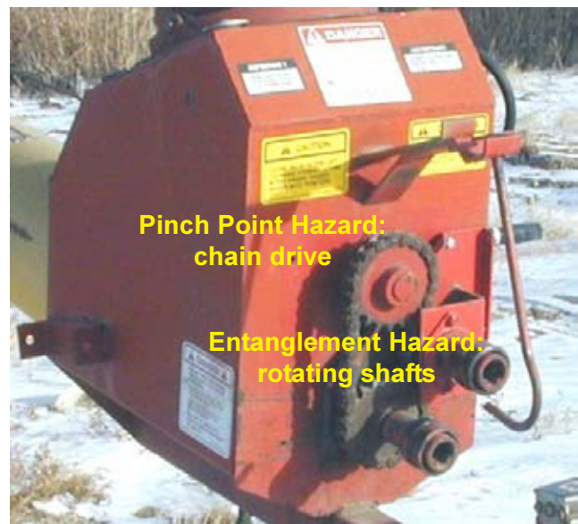
Figure 3. Chains, belts, and shaft drives are common hazards found on augers.
