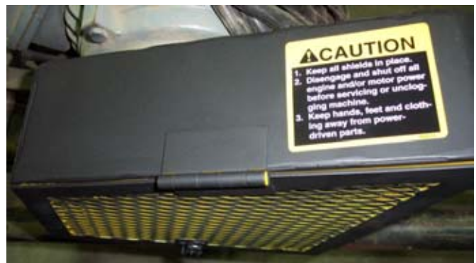
Figure 47. Safety decal installed.
