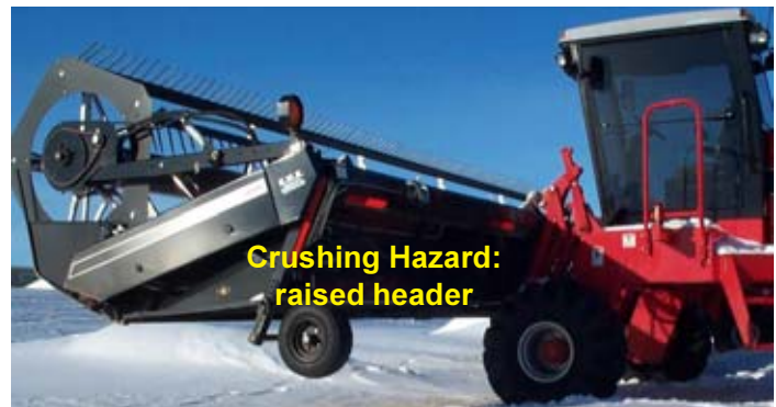
Figure 14. The crushing hazard under raised headers can be eliminated by using hydraulic cylinder stops.
