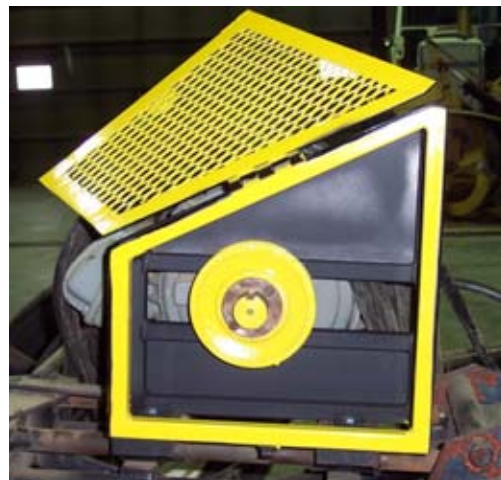
Figure 46. The inside of the guard and hazardous components were painted.
