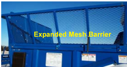
Figure 35. This expanded mesh barrier keeps people at a safe distance away from the rotating flails of a bale processor.
