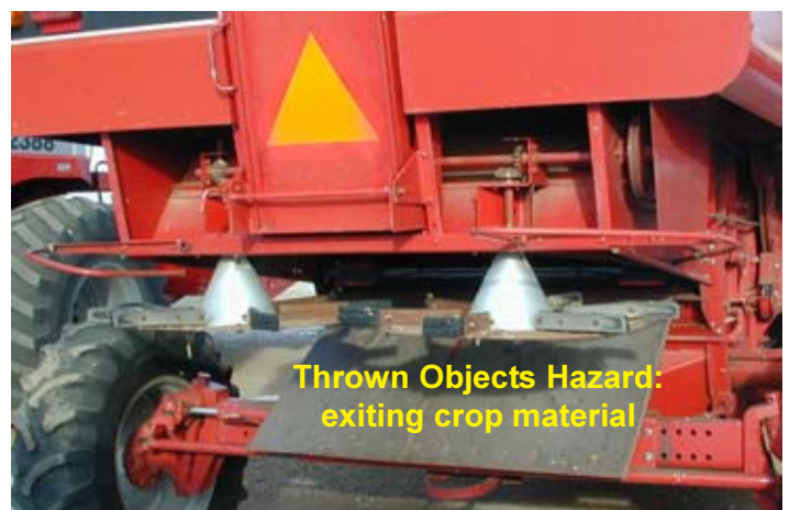
Figure 10. Combine choppers and spreaders can be hazardous because of crop material or objects that become airborne.
