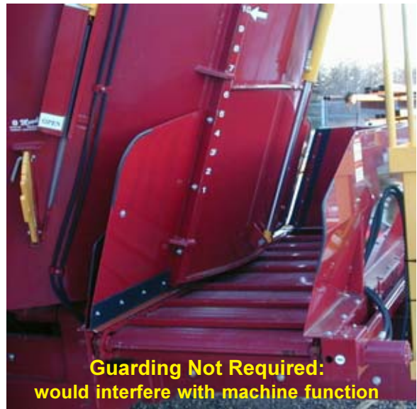
Figure 54. A guard is not required at the discharge of this feed mixer as it would interfere with the function of the machine.
