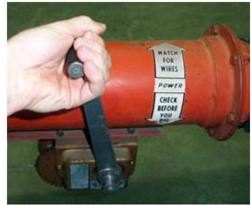
Figure 41. The over-head wire safety decals were located near the hand winch and near the auger inlet.
