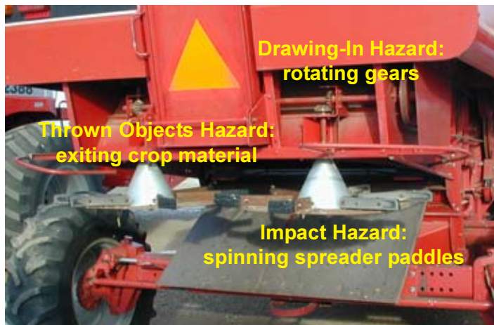
Figure 13. The rear discharge area of combines have multiple danger zones.
