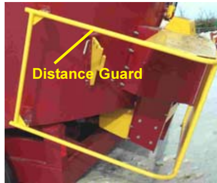
Figure 36. The distance guard on this feed processor keeps workers at a safe distance from the rotating knives when the cover is open.
