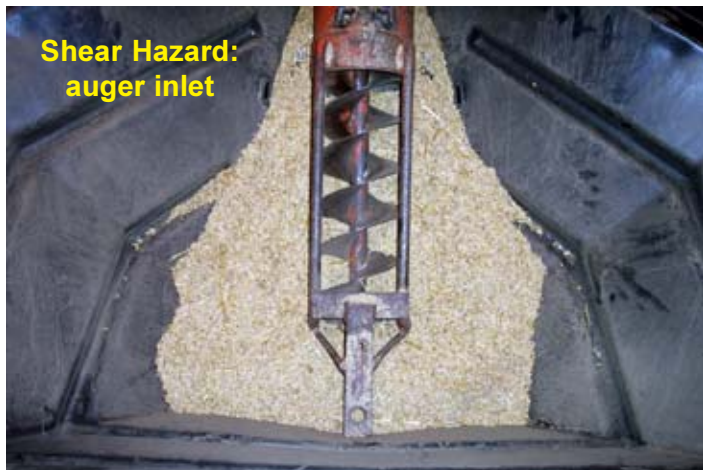
Figure 12. Auger inlets are often left unguarded.
