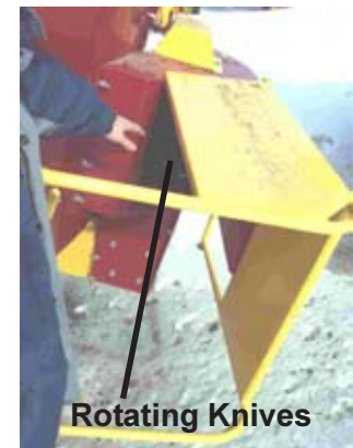
Figure 37. The worker cannot reach into the danger zone.
