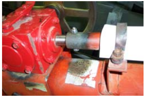
Figure 40. The exposed drive shaft.
