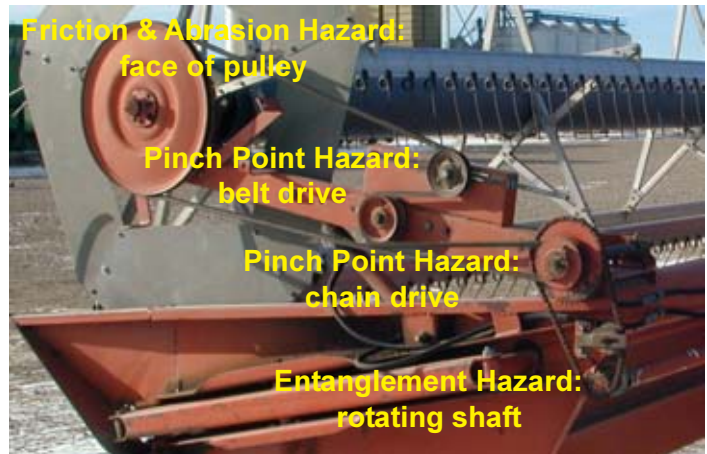
Figure 16. The header drives of windrowers are often left unguarded.
