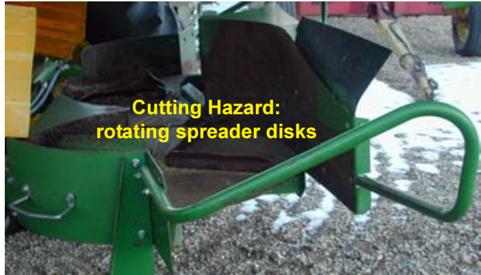
Figure 11. The spinning spreader discs of combines should have a distance guard similar to the one in this picture.
