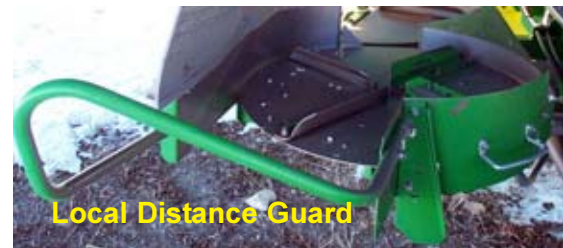
Figure 21. An enclosing guard would interfere with the function of this combine spreader disc.
