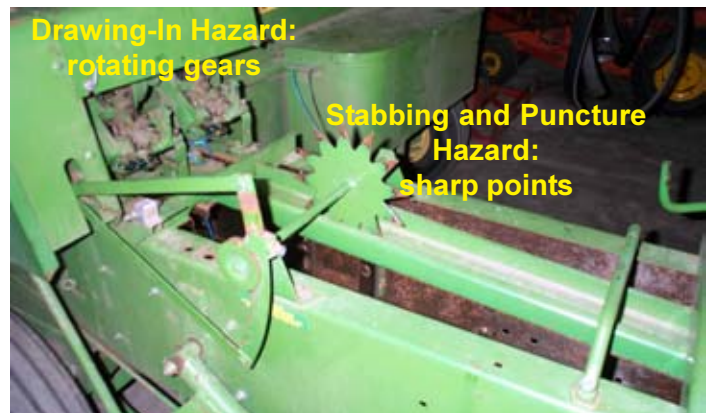
Figure 15. Sharp edges like the ones on this square baler are a stabbing or puncture hazard.
