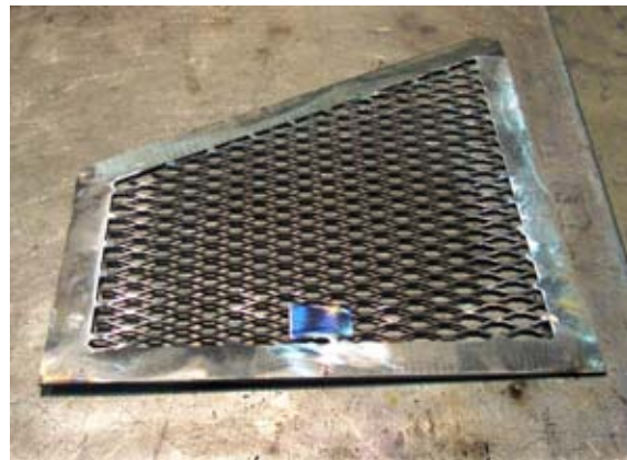
Figure 43. The expanded mesh door before installation.
