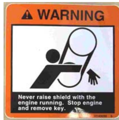
Figure 25. A safety decal warning of a pinch point hazard from a belt drive.
