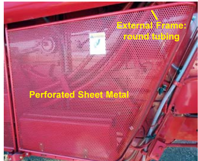
Figure 34. This perforated sheet metal guard provides protection from all sides and allows viewing of the hazard without opening the guard.
