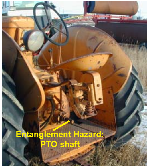
Figure 4. Guards for PTO shafts are commonly removed and not replaced.
