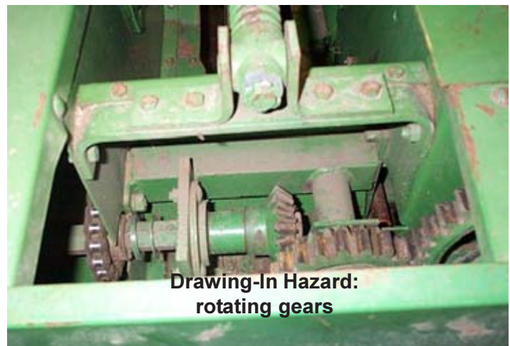
Figure 8. Loose clothing could be drawn in by these gears on a square baler.
