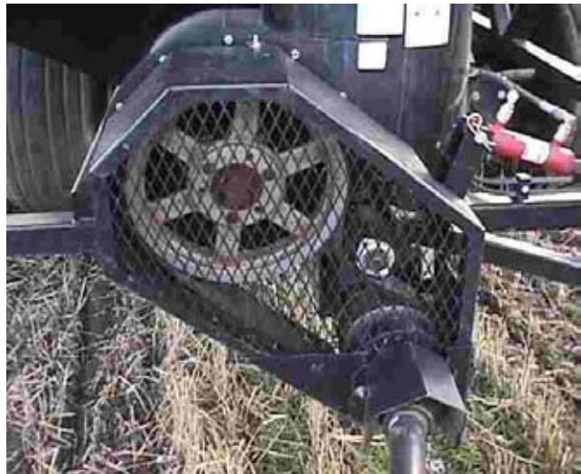
Figure 33. An Expanded Mesh Guard like the one on this grain cart allows viewing of the hazard without removal of the guard.
