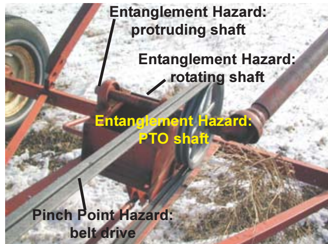
Figure 6. This PTO auger has multiple hazards associated with it.
