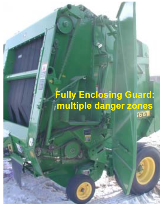
Figure 22. One fully enclosing guard can often eliminate multiple danger zones like on this round baler.
