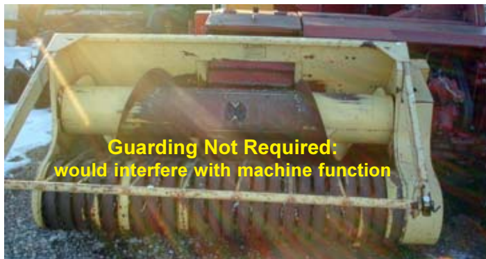
Figure 55. A guard is not required at the inlet of this forage harvester as it would interfere with the feeding of material.
