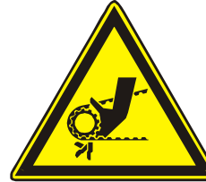
Pinch Point Hazard
