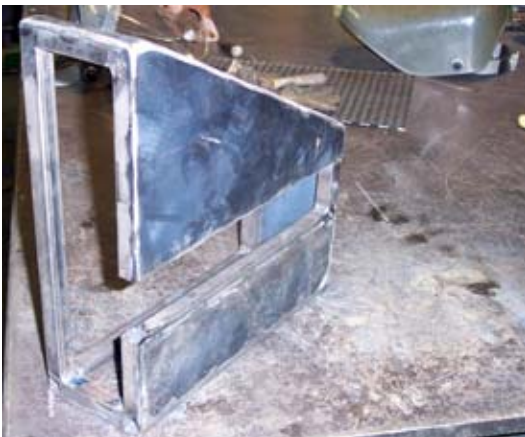
Figure 42. The sheet metal walls.
